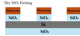
Fig. 5: Dry Etching of \text{SiO}_2 Layer
