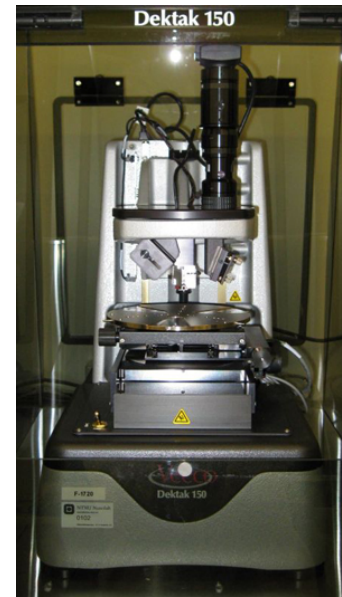
Fig. 10: Veeco Dektak 150 stylus profilometer used for surface topography measurements.
