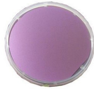
Fig. 9: Silicon wafer with thermally grown silicon dioxide layer prior to processing.
